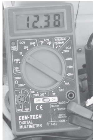
Voltmeter showing battery voltage reading
