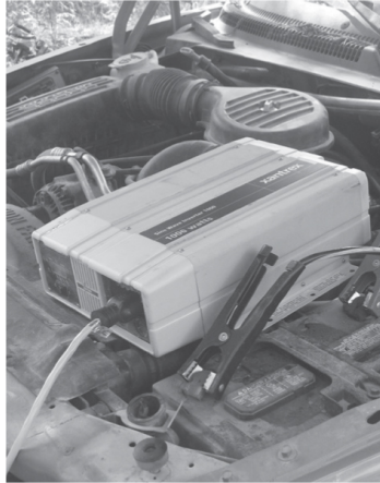
Inverter cables connected to car battery
