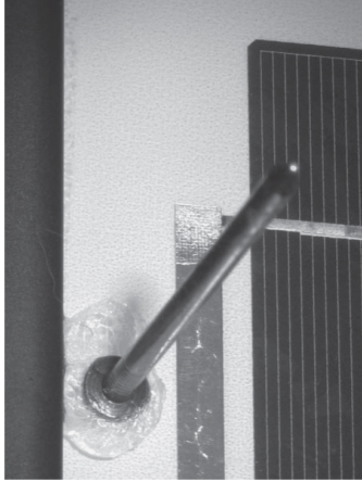
An example of using the nail test to correctly angle a panel
